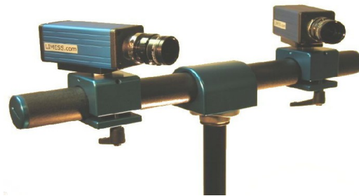
Figure 2: Stereoscopic setup for 3D-deformation measurement.
