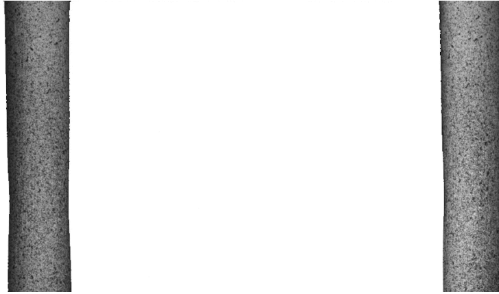
Figure 8: Images of a metal fastener before loading (left) and close before failure.
