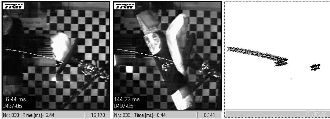
Figure 3: First and last image of the sequence with visualized tracking lines. In the 3. image the positions of the pattern are visualized.
